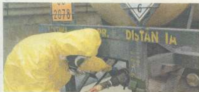
Personal protective equipment being used during the unloading of TDI from a tanker.
